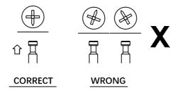
When fitting cam lock, ensure starting position is correct before you insert connecting quickfit.
